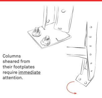
Twisted columns are difficult to assess. Horizontal and diagonal braces are essential to the capacity and stability They may impede the load capacity of of the rack system. Any missing, the rack, which is why we recommend detached or torn braces should be calling an expert.
