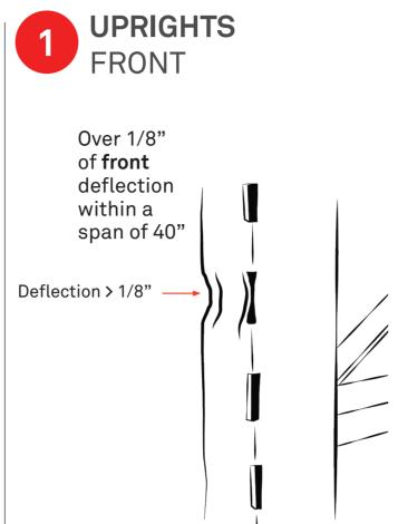
Also look for other types of damage such as dents, cracks, bulges, pinched columns and signs of corrosion.
