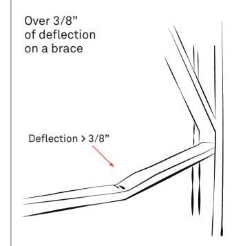
Also look for cracked or broken welds between the column and the brace.
