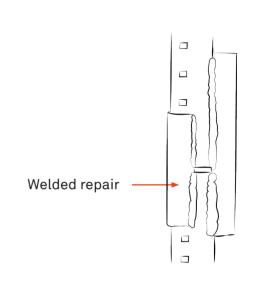
Unless approved by an engineer, any home made repair should be replaced by an engineered repair solution. Welded splices and non-matching extensions are signs of local repairs.
