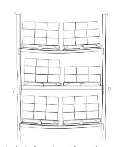
Labels informing of maximum load capacity should be visible and easily read by all. If you don't know the load capacity of the racks, it should be determined by a Professional Engineer.
