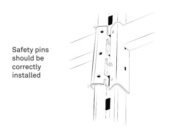
Look for corrosion, deformations, cracks in the welds, broken connectors and/or missing safety pins. Safety pins are essential to prevent beam clips from detaching.
