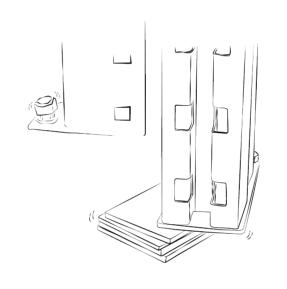
Look for missing, loose and/or damaged anchors or foot plates. Shims should be well seated, well secured and of equal size to the footplate.
